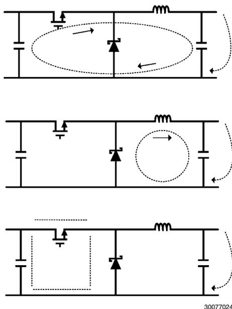
**FIGURE 4. Current Flow in a Buck Application**
